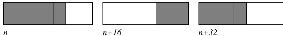
Figure 4. Example of machine instructions aligned to 16-byte blocks. NOP padding is shown in white. Call instructions are placed at the end of 16-byte blocks, so that return instructions will jump to the start of the next block.
